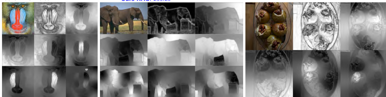
Fig. 6. Some of the 50 eigenvectors of a simple pixel affinity matrix extracted with our multiscale solver.
